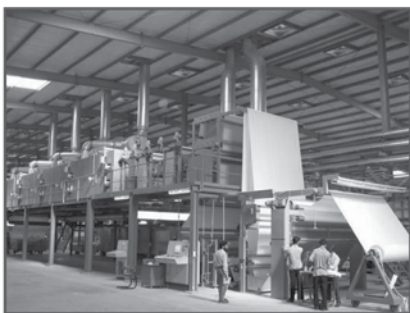
Figure 3: POWER-COLORTHERM / INFRATHERM Pad-Dry / Thermosol lines ensure an optimum dyeing and a crease-free fabric passage
